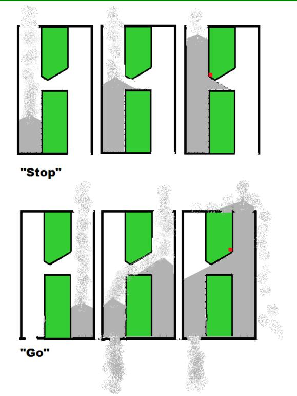
Note the red dots ( ) for each application. This is where the angle of repose STARTS!
